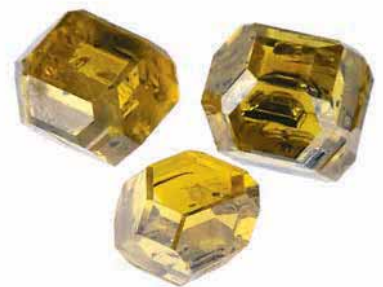
ABOVE: Synthetic diamond crystals grown from a metal flux at HPHT
